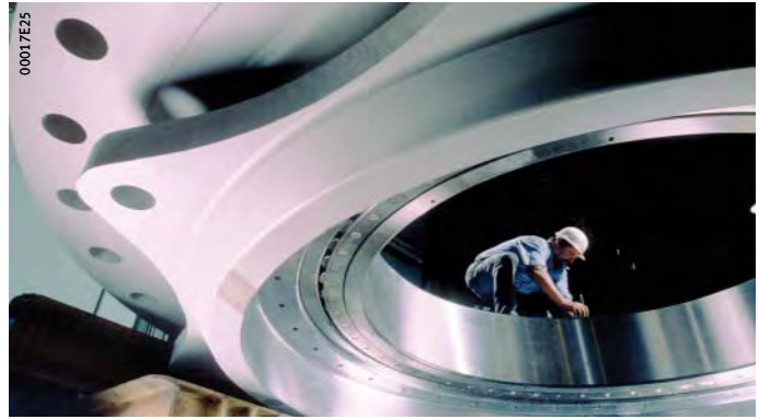
Figure 3 Mounting of a large rolling bearing
