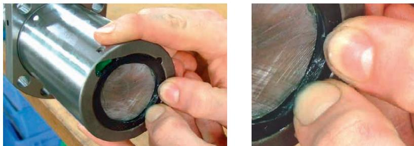
Fig. 4.7 Fixing the wiper while slowly screwing nut onto shaft
