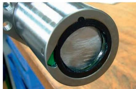
Fig. 4.6 Screw nut with wiper onto shaft
