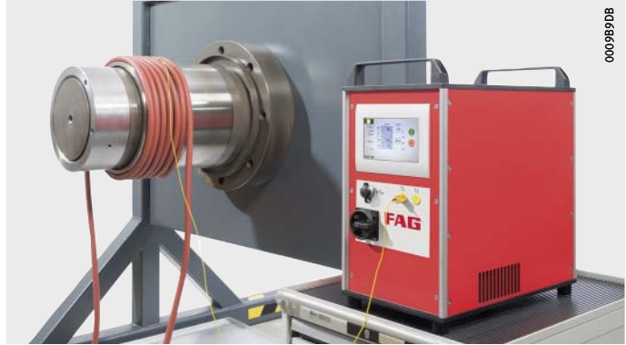
Figure 2 Induction heating of inner ring
